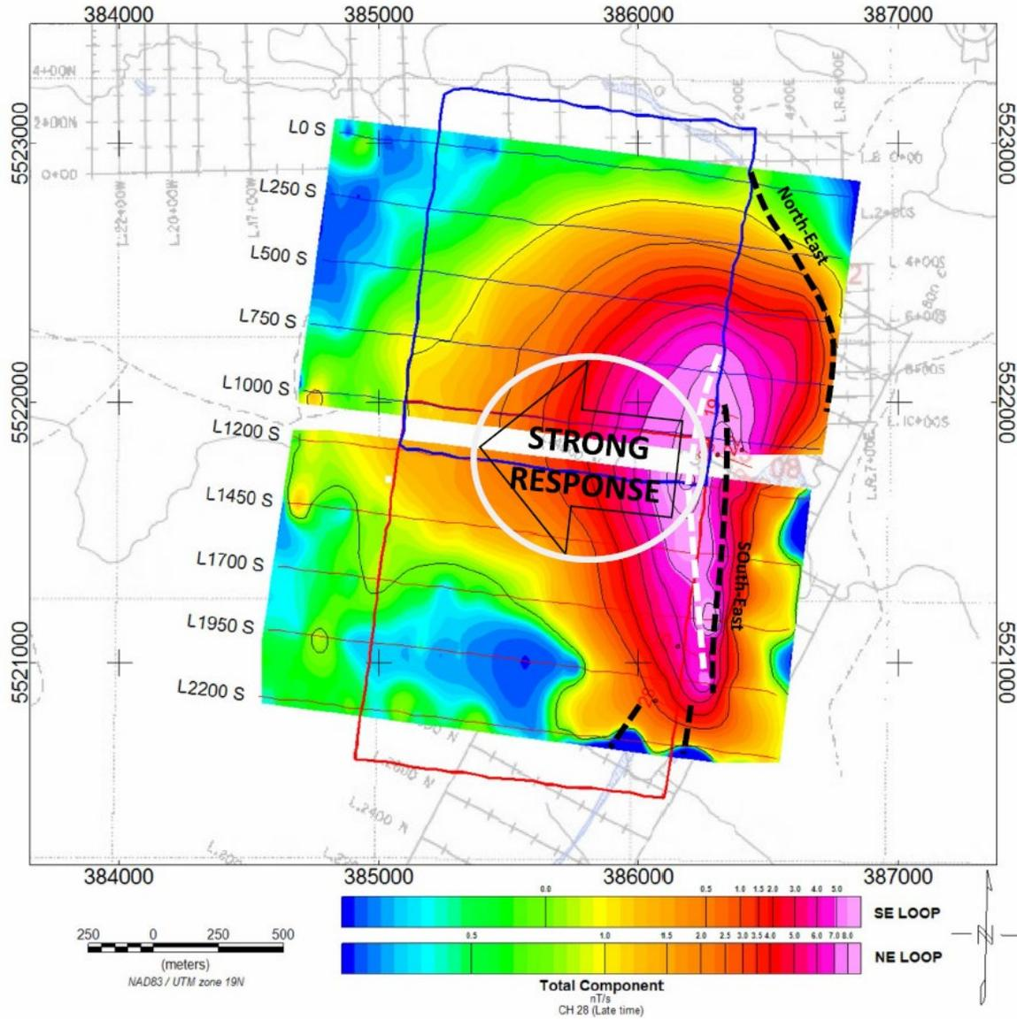
Figure 15: “Latest-time” response showing strong response which indicates the size and trend of the anomaly.
