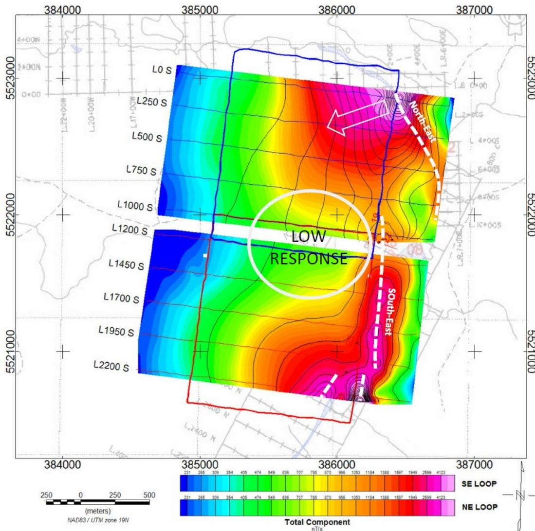
Figure 13: “Early-time” response showing the low response in the center, indicating a thickness to the zone.
