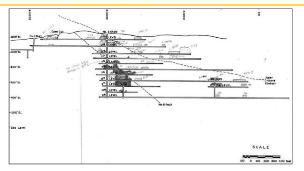
Figure 8: Section W-E showing the underground works at Castle Mine
