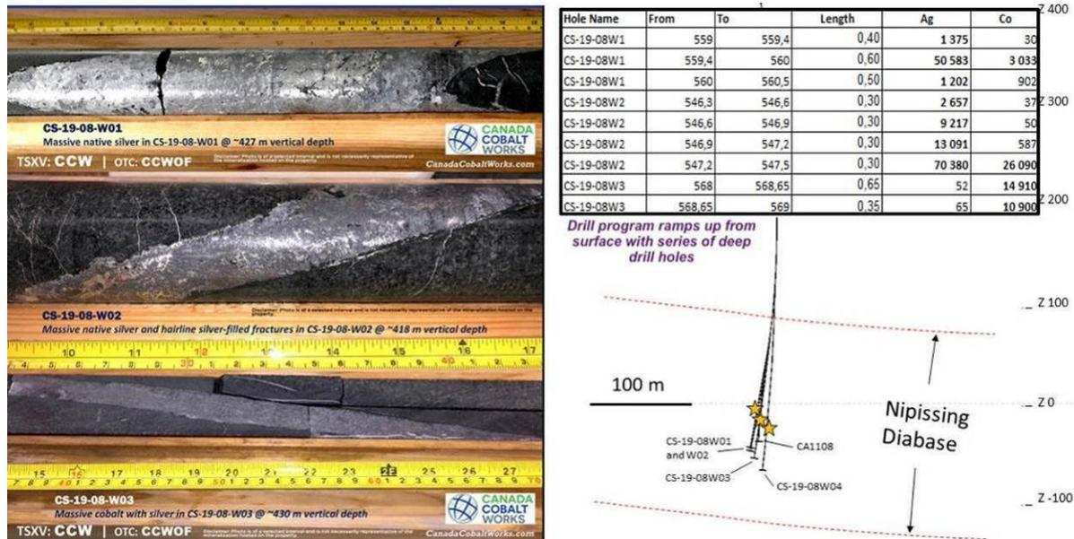
**Figure 54: Massive silver mineralisation in hole CS-19-08 W01, -W02 and -W04 with vertical section showing the thickness of the Nipissing diabase**
