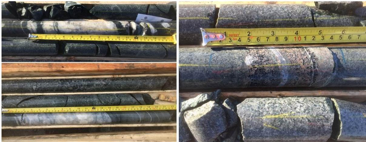
**Figure 15: Drill core with veins mostly filled by quartz cements within the Nipissing diabase**
