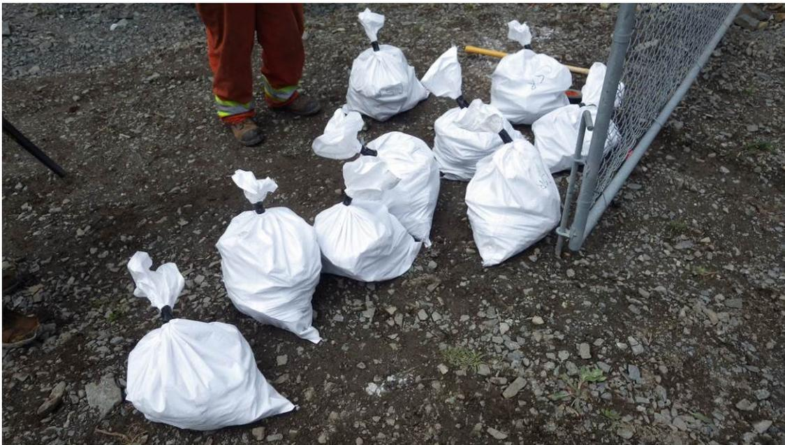
**Figure 59: Core samples in rice bags ready to ship to the laboratory**
