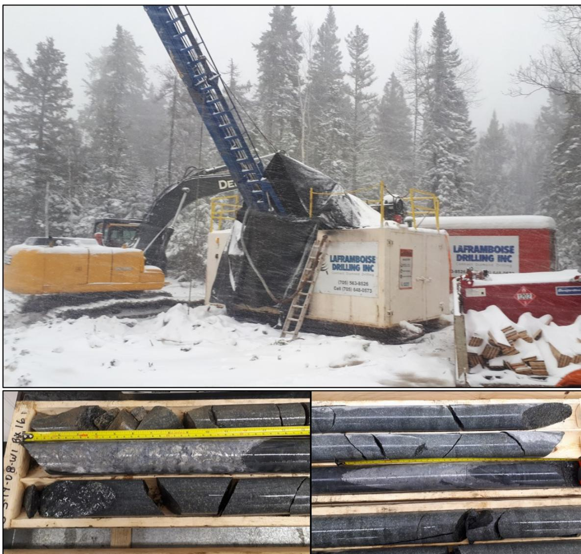
**Figure 55: Drilling program 2019/2020, with drill core showing massive silver mineralisation**
