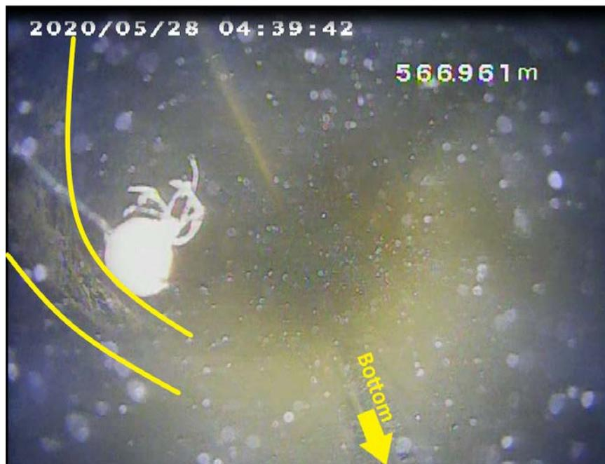
**Figure 39: Vein contact at 566.961 m (measured by the depth sensor)**
