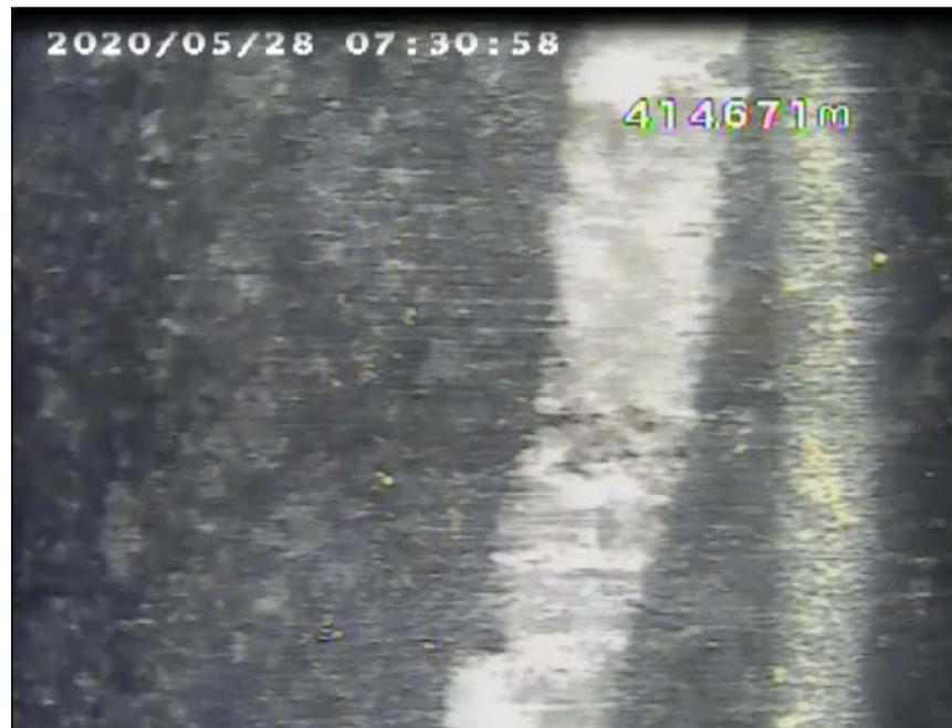
**Figure 38: Vein in lateral view at 414.671 m (measured by the depth sensor)**
