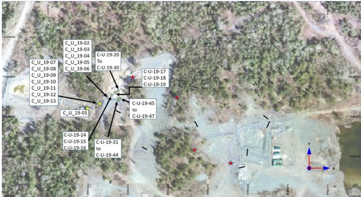
**Figure 42: Location of the underground drill holes program 2019.**
