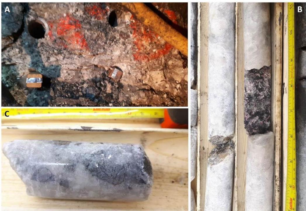
**Figure 46: A) Showing collars marked using a labelled wood piece; B) Drill hole following the quartz vein; C) Core showing silver and cobalt-arsenides mineralisation**
