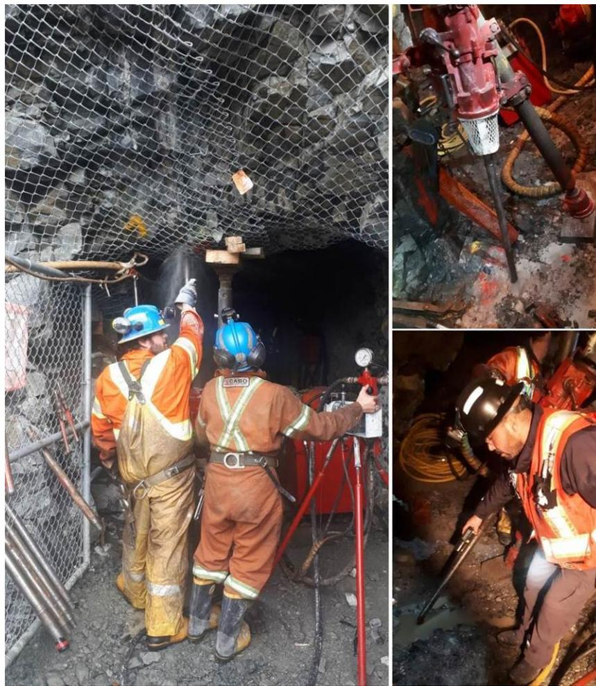
**Figure 44: Underground drilling with electrical drill (drill size AQ)**
