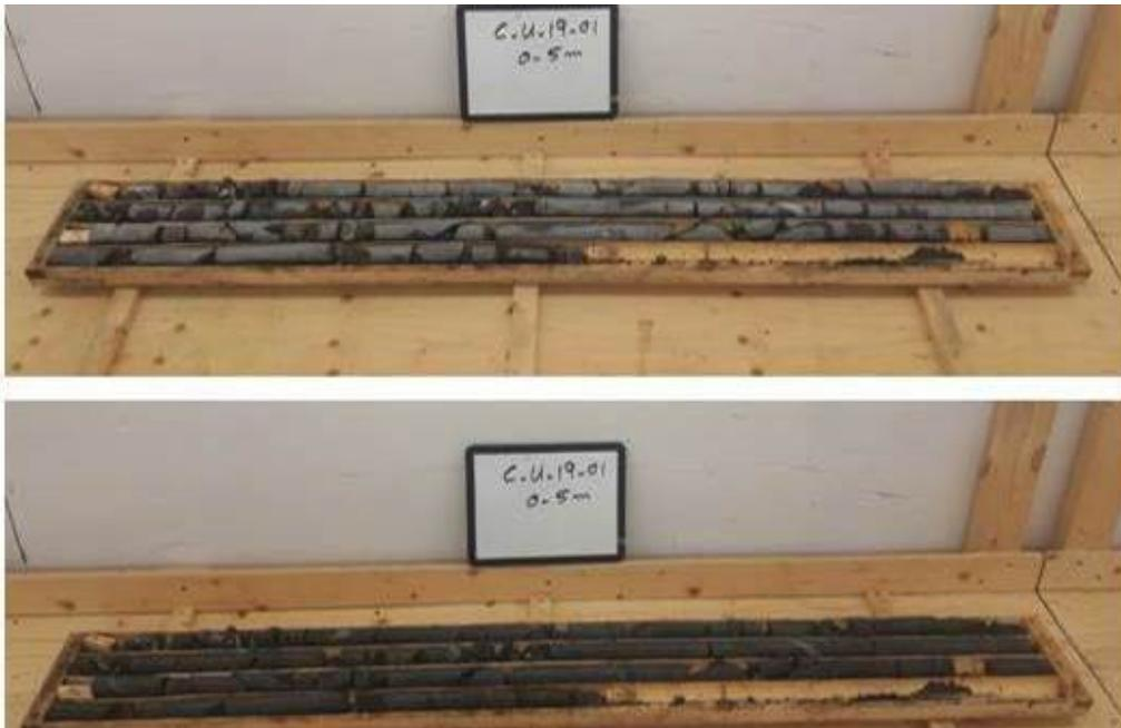
**Figure 45: Photos of dry and wet core taken from hole C-U-19-01**
