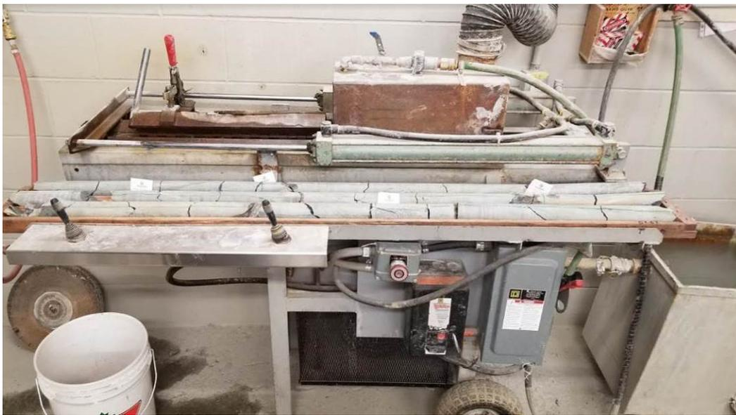
**Figure 57: Electrical saw used for cutting the core samples**
