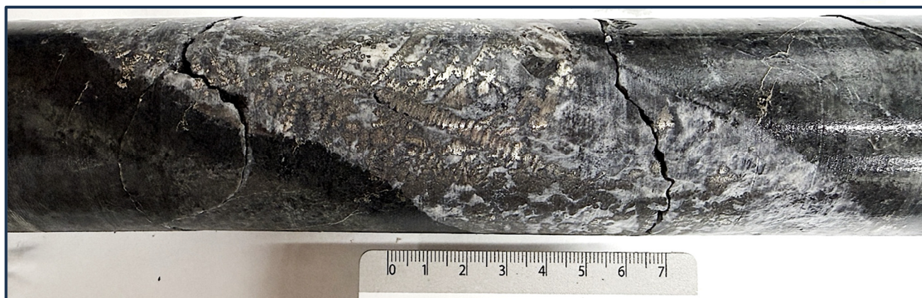
Figure 1: Picture of new intersection Interval from hole CS-21-73W1 grading 61,389 g/t silver over 0.3m and 2,848 g/t silver over 6.65m.
