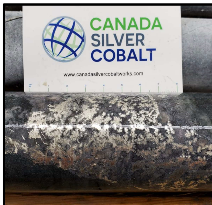
Figure 4: High-grade silver mineralization over 5 – 7 cm true width in hole CS-20-39 with a spectacular 89,853 g/t Ag (2,621 oz/Ton) over 0.3m from 557.46 – 557.76m; comparable to the average thickness of veins that produced over 65 million ounces from the 3 major past-producers within 2 km of the Robinson Zone.
