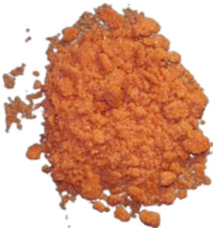
Fig. 4: Cobalt sulphate produced from Castle Mine concentrate using the re-2Ox process
