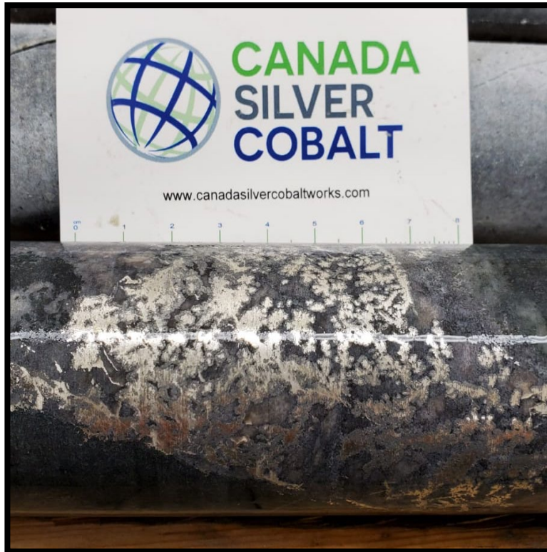
Figure 4: High-grade silver mineralization over 5 – 7 cm true width in hole CS-20-39 with a spectacular 89,853 g/t Ag (2,621 oz/Ton) over 0.3m from 557.46 – 557.76m; comparable to the average thickness of veins that produced over 65 million ounces from the 3 major past-producers within 2 km of the Robinson Zone.
