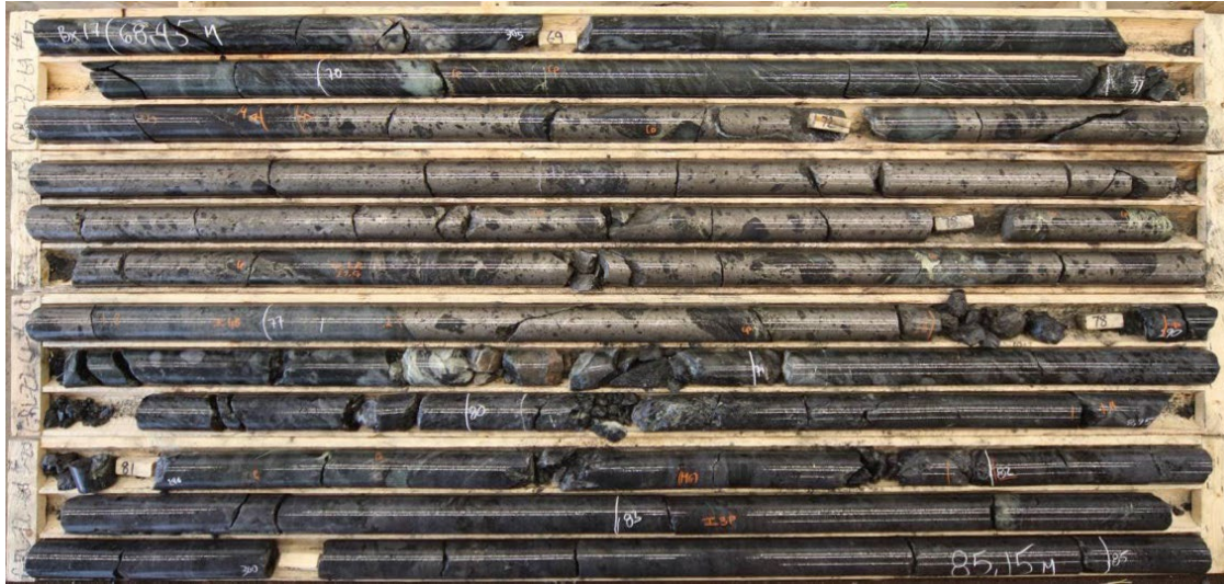
Figure 6: Core photo of GRL-22-61, highlighting the sulphide intersection between 62.10 to 77.80m (News Release February 16, 2023)
